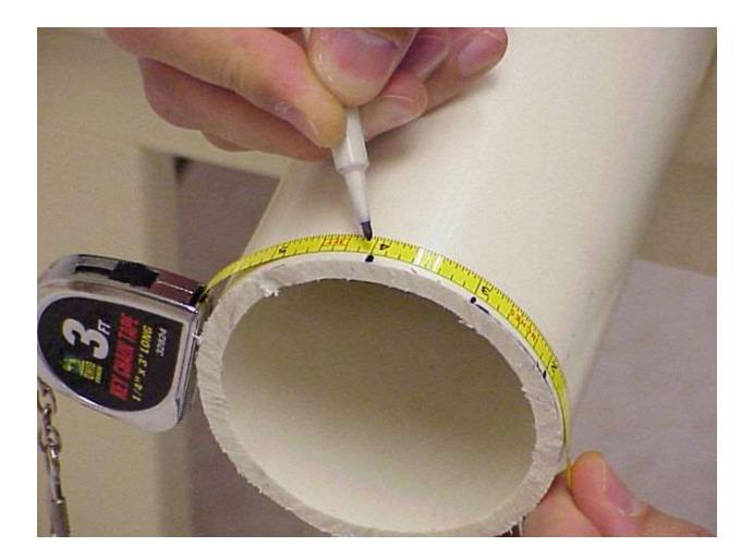
At each mark, draw a line  $\frac{1}{2}$  inch down the tube (picture 2). This will be the depth of the teeth.
