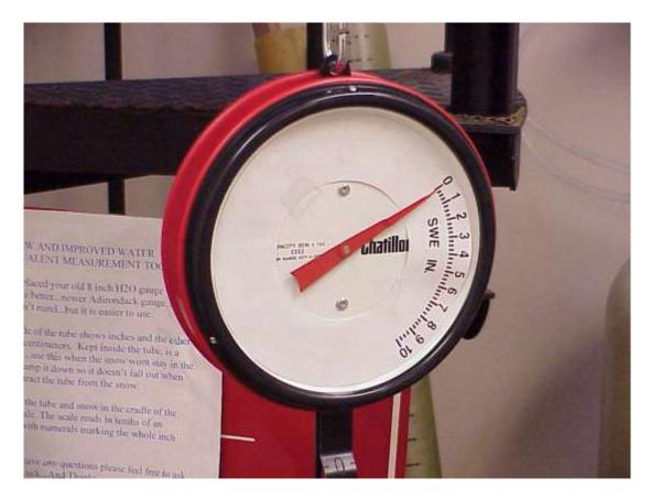
Most scales have an adjustment screw on the hanger to fine tune the zero reading. Read the instructions with your unit.
