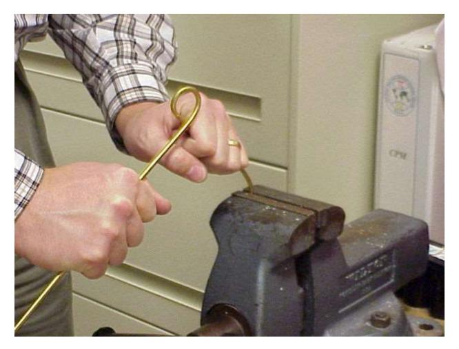
Measure 10" in from each end, and bend the rods so that when you hold the rod by the loop in the middle, the bent rod ends point straight down.
