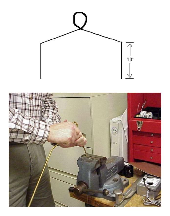
Bend the rod ends into a half circle, large enough to hold the PVC pipe. As an option, you can slip a length of 3/16" clear vinyl tube over the ends to add a non-skid surface. The 2 inch hook is used to attach the hanger to the scale.
