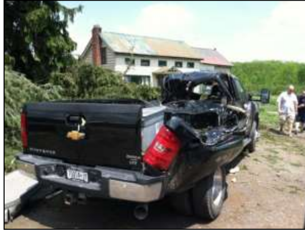
Figure 2: Truck destroyed at 451 South Shore Rd. in Mariaville. A wooden board was driven into the truck below the rear windshield. Photo Source: NWS Albany
