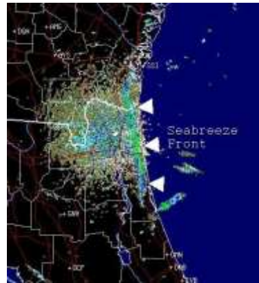
Figure 2. Radar Depiction of a sea breeze front along the coasts of Northern Florida and southern Georgia. Sea breeze fronts strengthen and move inland during the day, and weaken and retreat in the evening. Image courtesy of NWS Jacksonville, FL.
