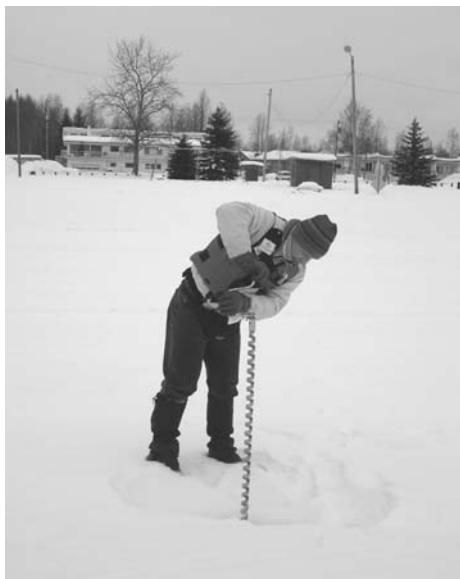
Dave Streubel prepares to take an ice thickness measurement on Lake Hood
