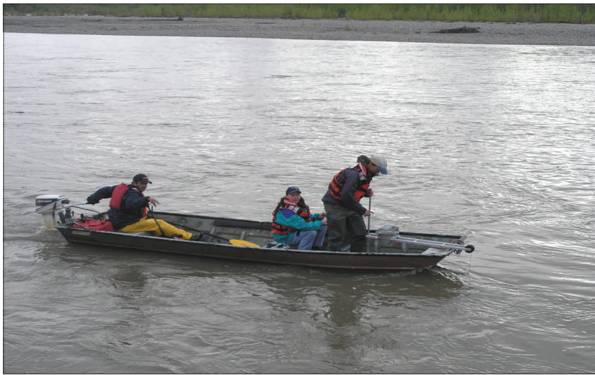
RFC Hydro Tech Becky Perry and Fairbanks WFO Service Hydrologist Ed Plumb take a flow measurement on the Koyukuk River at Bettles. Local resident Tom Shanahan drove the boat.
