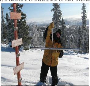
Ben Kennedy (BLM) measures the weight of a snow core in order to determine the amount of water in the snowpack.
