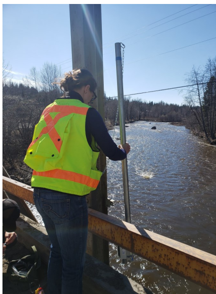
Figure 1: Senior Service Hydrologist Celine van Breukelen installing an automated gage on the Anchor River. Picture: NWS staff.
