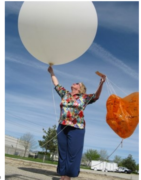
NWS Boise employee, Valerie Mills, launches weather balloon and radiosonde
