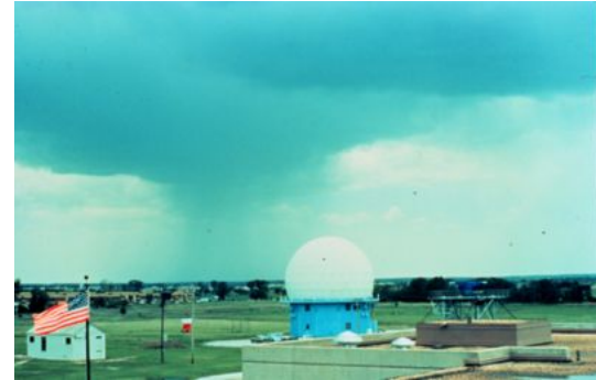
Doppler Weather Radar in Norman, OK with a rain shaft in the background.
