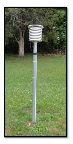
Pictured left is a sensor on a galvanized pole. Pictured below is a Nimbus readout display which always displays the current temperature.
