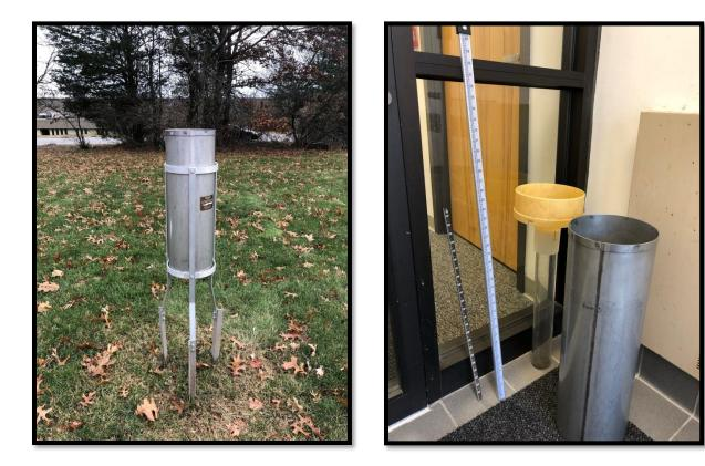
Pictured above left is the SRG ready for winter time precipitation as the inner tube and funnel have been removed and placed inside. Pictured above right are the tools needed for snow operations. There is the spare overflow can for swapping out. There is the inner tube, funnel and precipitation stick for measuring the melted wintry precipitation. And finally there is the snow stick for measuring snowfall and snow depth.
