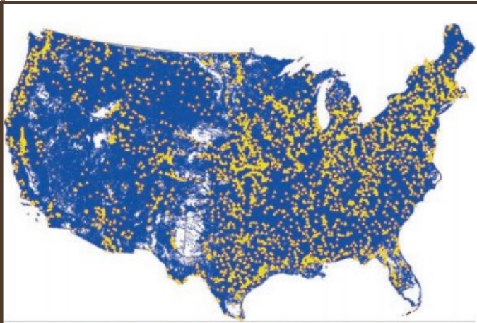
National Water Model provides many more locations nationwide with streamflow forecasts (blue) than the current Advanced Hydrologic Prediction Services of only about 4,000 locations (yellow).
