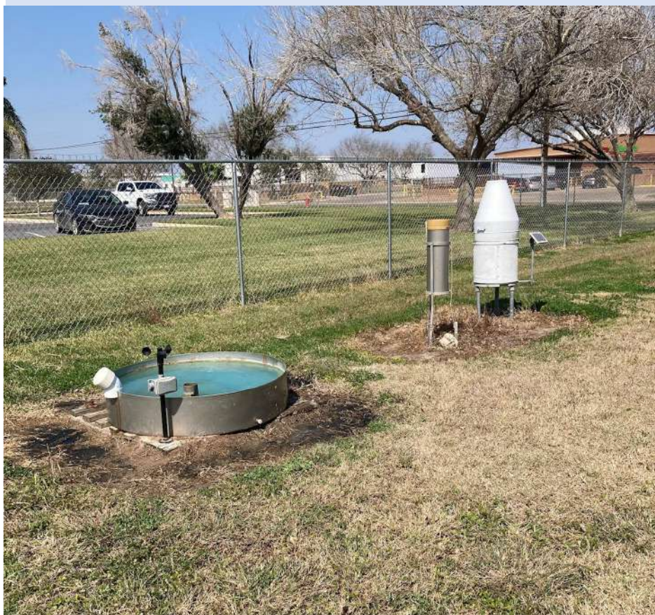
COOP Site with Evaporation Pan and Totalizing Anemometer, 8" Standard and Fisher Porter rain gauges.
