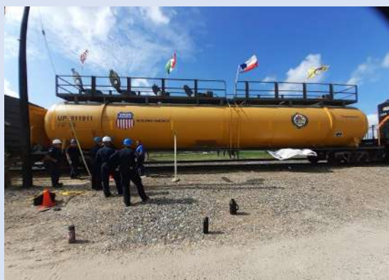
Tank Car designed to carry compressed or liquid commodities, like chemicals, molasses, edible tallow, water, and diesel fuel. Multiple types of fittings can be seen on the top which are used for demonstration purposes. Photo by Brian Miller
