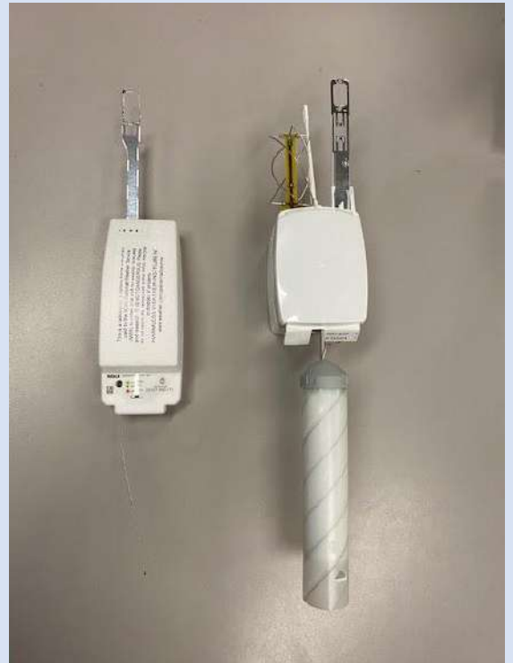
Pictured Above: New RS41 Radiosonde (left) vs old RS92 Radiosonde (Right). Pictured Below: New Antenna. Photos by Amber McGinnis
