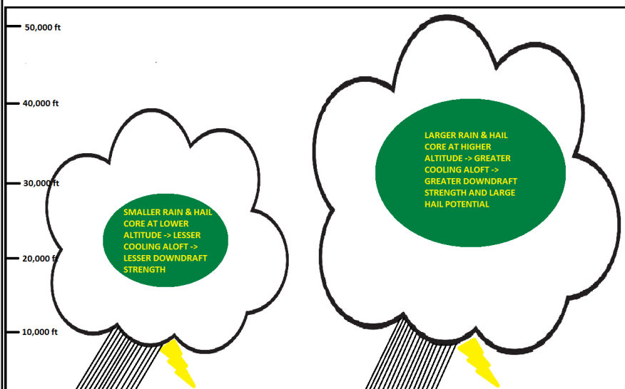
Figure 3. Illustration of downward mass transport within a pulse thunderstorm. A larger and higher mass of precipitation within a storm will lead to a greater potential of severe downdraft winds and large hail.
