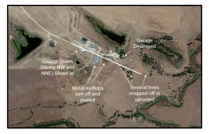
There was considerable damage to buildings on a local ranch. A shop building had 2 doors blown in and roof damage. Two other sheds had significant roof damage. Several metal rooftops were torn off and peeled back. A small garage was destroyed with a vehicle displaced inside, turned and moved by a couple feet. Several trees were snapped (approximately 1 foot diameter), with other smaller trees blown over or uprooted.
