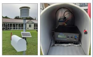
This site on runs off of solar energy that charges a battery and connects to the temperature readout. The solar panel method is more energy efficient and allows for more accurate readings each day. The temperature display is called a NIMBUS and can save up to a month worth of daily observations.
