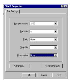
Click on Configure and choose port settings at the desired baud rate (300,1200,2400,9600, or 19200). Then select eight data bits, no parity, one stop bit, and no flow control. Then click OK. At this point the window will vanish, but with additional setup required click on File|Properties:
