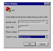
Choose "Connect Using" whatever comport is connected to your external serial port. Here we have chosen Com2. Click [OK] and then click on the settings tab.
