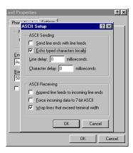
Select Echo typed characters and click the OK button to close the windows. The program is now set up to communicate with the Nimbus PL Thermometer. The command set may be retrieved using command at?
