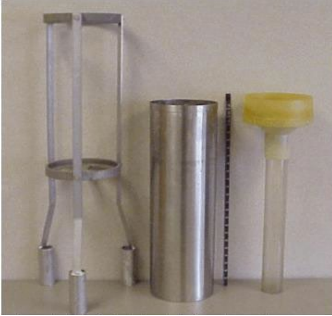
Figure A-4. Eight-Inch Precipitation Gauge Components
