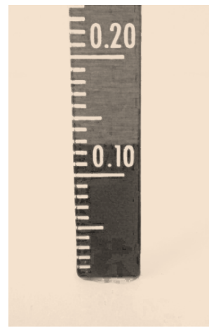
Figure B-13. Reading the Precipitation Amount (0.13)
