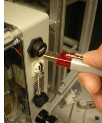
Figure B-24. Insert Flash Drive to Download Data
