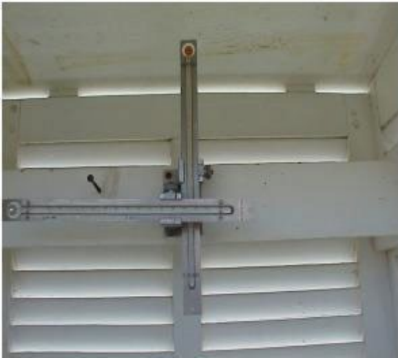
Figure B-29. Minimum Thermometer – Vertical Position During Resetting
