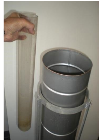
Figure B-10. Removing the Measuring Tube
