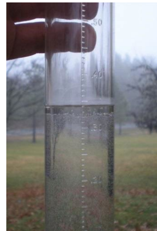
Figure B-7. Reading the Measuring Tube - Eye Level
