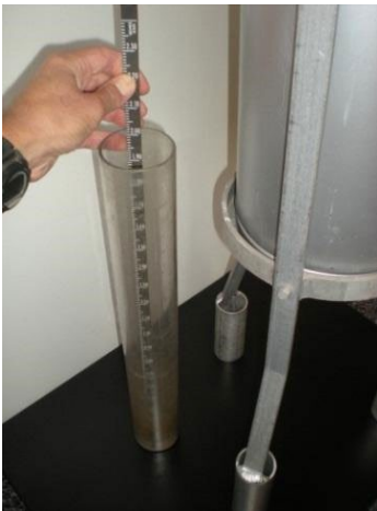
Figure B-11. Dipping the Measuring Stick
