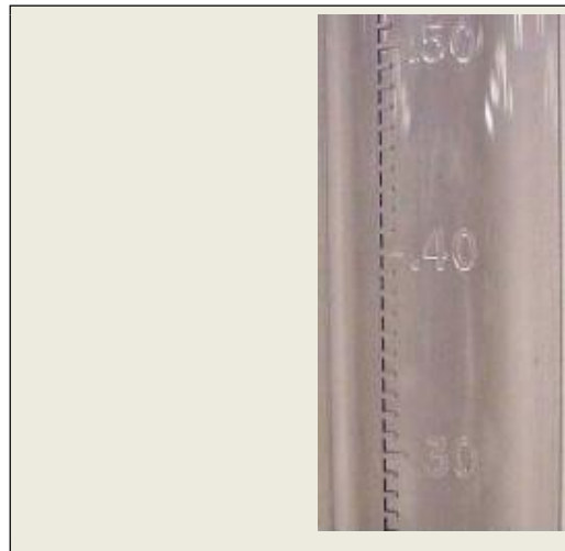
Figure A-7. Graduated Measuring Tube (Hundredths of an Inch)
