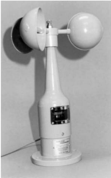
Figure A-26. Totalizing Anemometer with 6-Digits
