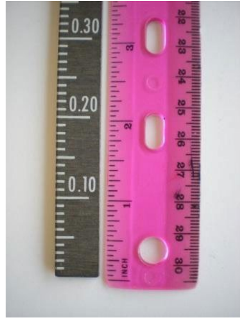
Figure A-5. The Measuring Stick (brown) for the Eight-Inch Gauge
