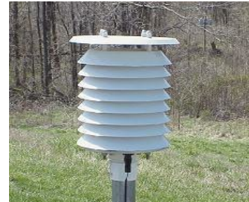
Figure A-13. MMTS Shelter
