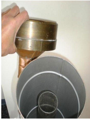
Figure B-9. Removing the Funnel
