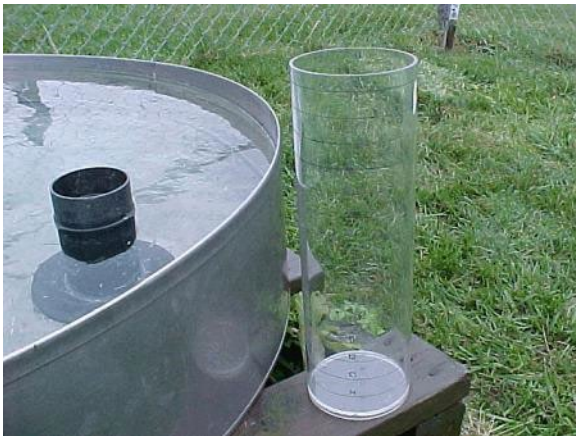
Figure B-35. Transparent Measuring Tube and Stilling Well Inside the Pan
