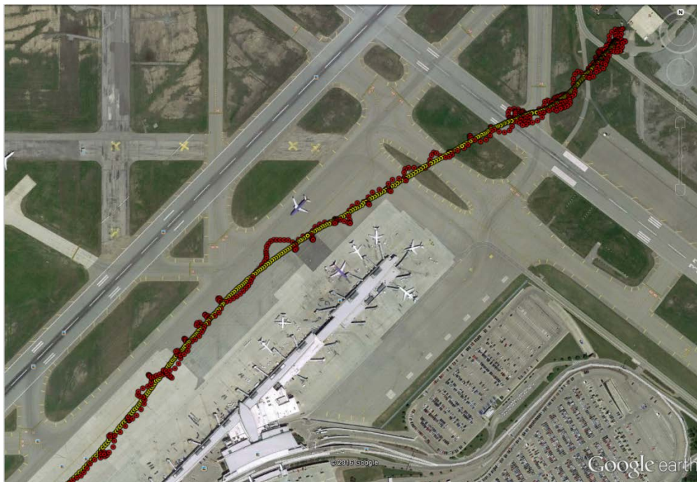
Figure 1. Unsmoothed (red dots) path actually taken by the radiosonde. Note the spiral path, which is due to the “pendulum” action of the radiosonde and flight train. The yellow dots represent the smoothed position.
