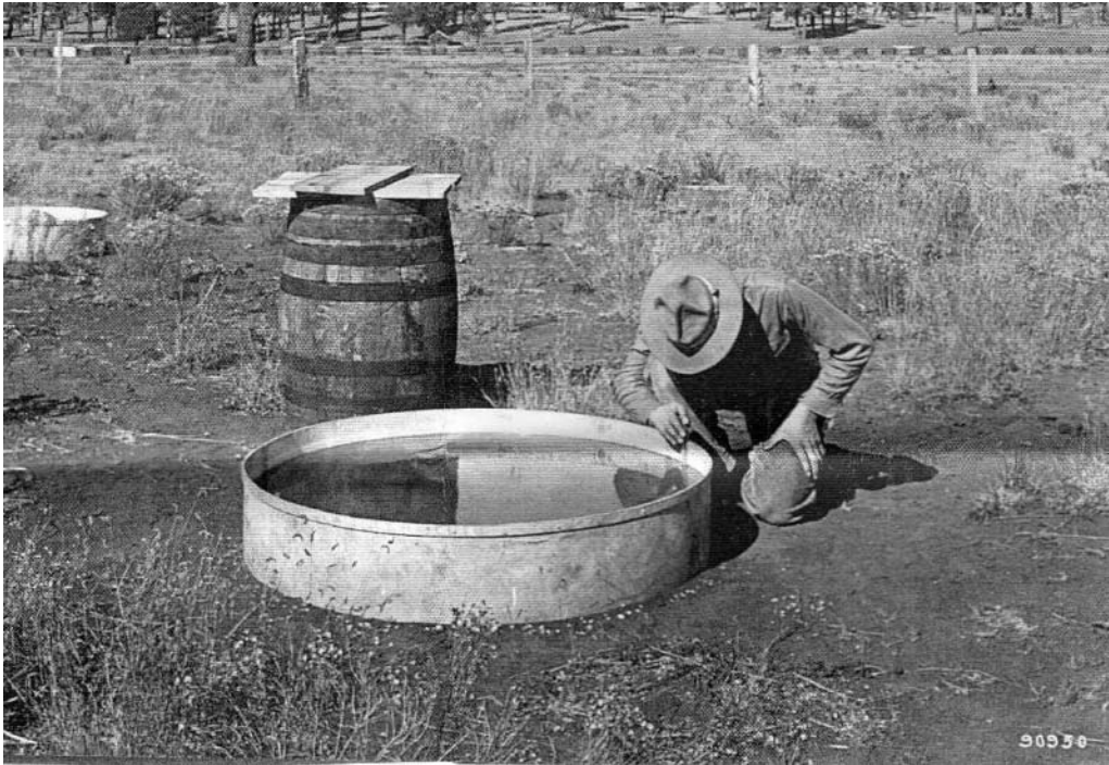
G. A. Pearson measuring water level in evaporation pan. Photo A. G. Varela, 1912. USFS photo # 90950
