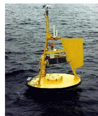
NOAA 3 meter discuss buoy in Casco Bay
