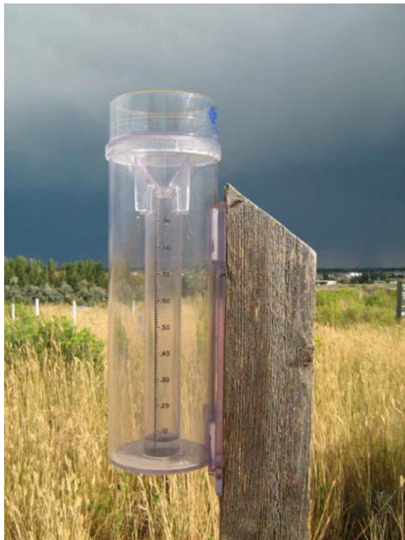
Figure 3: A well placed rain gauge is far from any obstructions (including trees and fences), 4 to 5 feet off the ground, and level.
