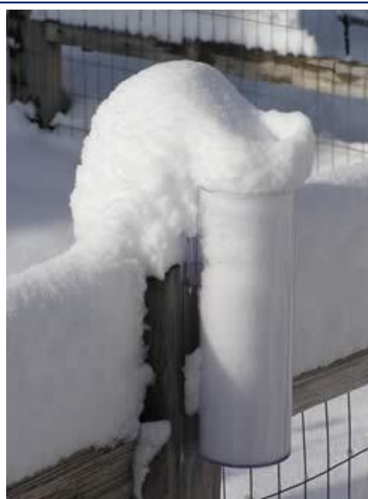
Figure 3: Snow measurement can be one of the hardest parts of weather observations. In this image, a traditional rain gage is buried in snow and would not provide an adequate measurement.
