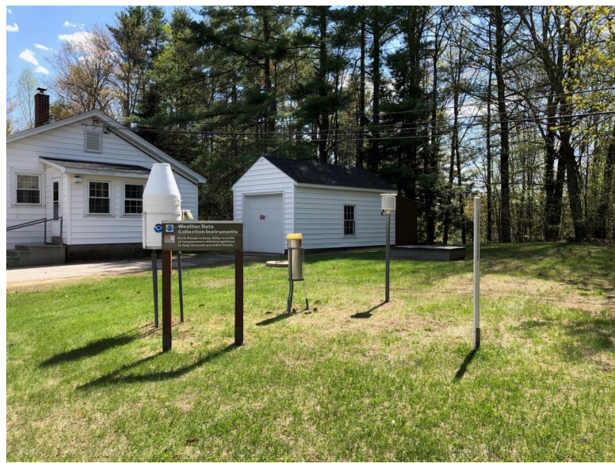
Figure 6: A typical Cooperative Observer station. These are often located at the homes or businesses of volunteer observers.
