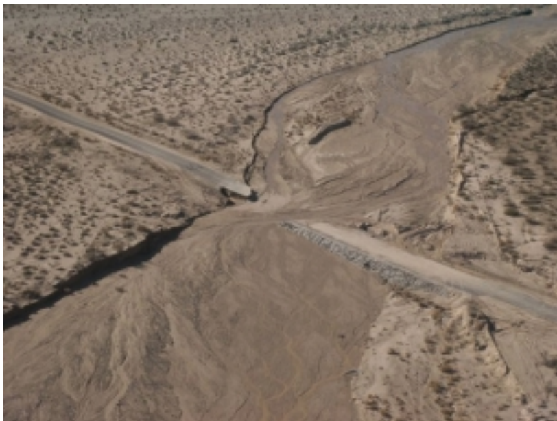
Aerial photograph compliments of WCM Dan Gudgel showing the Redrock-Randsburg Road in the Kern County Desert cut by flooding due very high 24-hour rainfall by the morning of January 10th.
