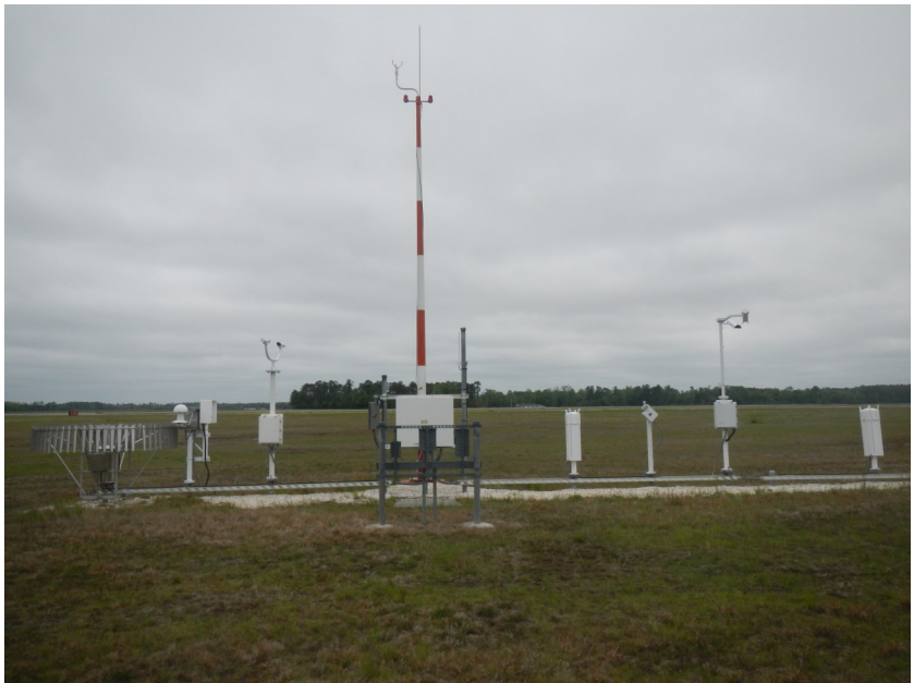
The Wilmington Automated Surface Observation Station (ASOS) which measures wind, weather, visibility, cloud height, temperature, rainfall, and many other meteorological variables!
