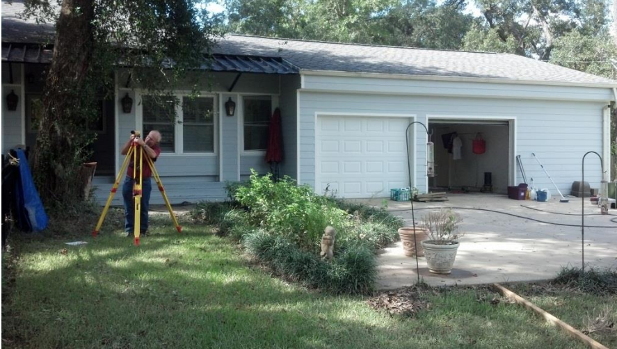
498 499 Figure 17. The Montgomery home on Magnolia Dr. had a clear high water mark inside of the 500 attached garage. Flood survey team members Marty Pope (pictured) and W. Scott Lincoln used 501 this high water mark to help estimate the crest for the Wolf River at Bells Ferry Rd. (GLFM6) 502 forecast point. 503
