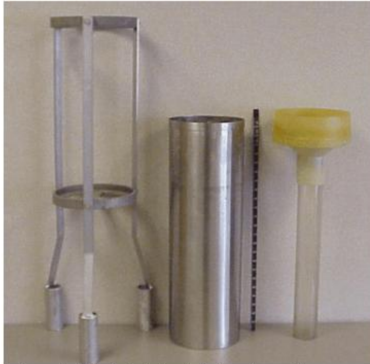
Figure A-4. Eight-Inch Precipitation Gauge Components
