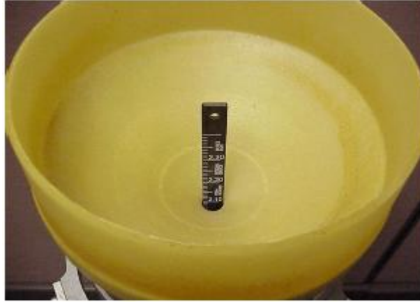
Figure A-30. Eight-Inch Gauge with Measuring Stick Inserted
