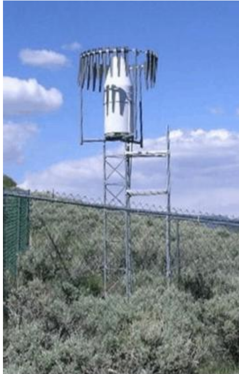
Figure A-3. Fischer & Porter Gauge Mounted on a Snow Tower with Wind Shield
