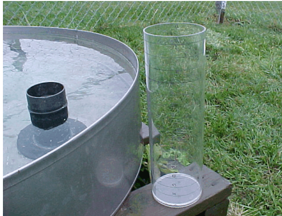
Figure D-4. Transparent Measuring Tube and Stilling Well Inside the Pan
