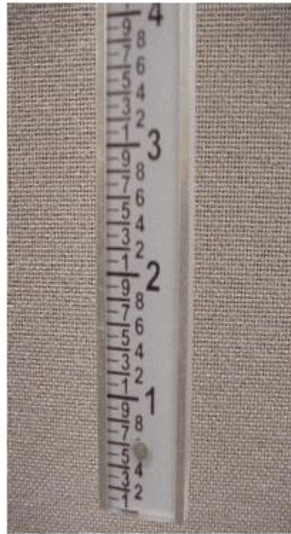
Figure A-33. Snow Stick Graduated Scale to a Tenth of an Inch
