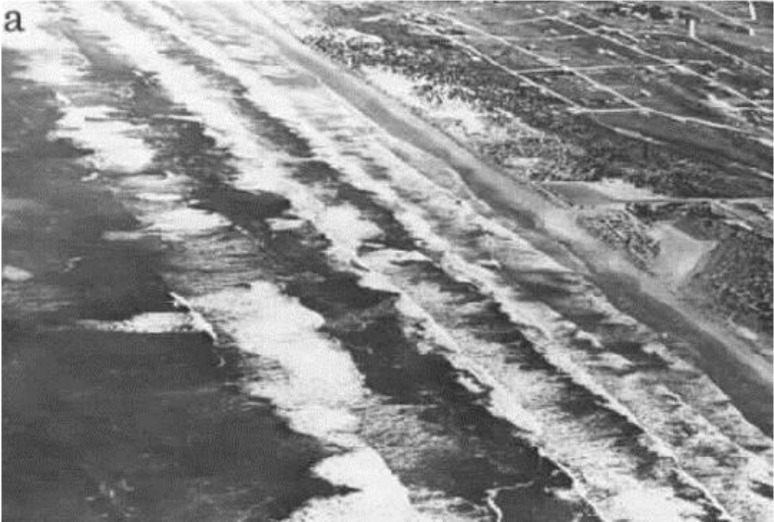
(A) Spilling breakers in series with saturated surf zones. Usually can be seen at low tide. Waves are high.
