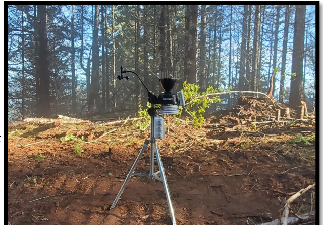
New rain gauge installed on the Tyee Complex burn scar in Douglas County
