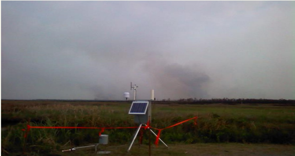
A portable RAWS station deployed on the Pain's Bay Fire in May 2011. This equipment provided additional observations of temperature, humidity and wind to the IMET, which resulted in more accurate forecasts. Photo by Jim Merrell
