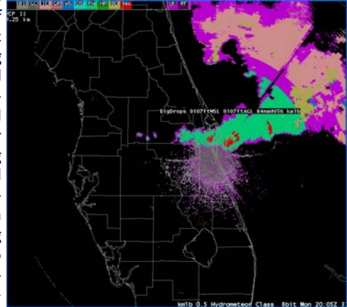
Fig 3. Sample radar image from KMLB (Melbourne, FL) displaying Hydrometeor Classification from a dual polarimetric radar.
