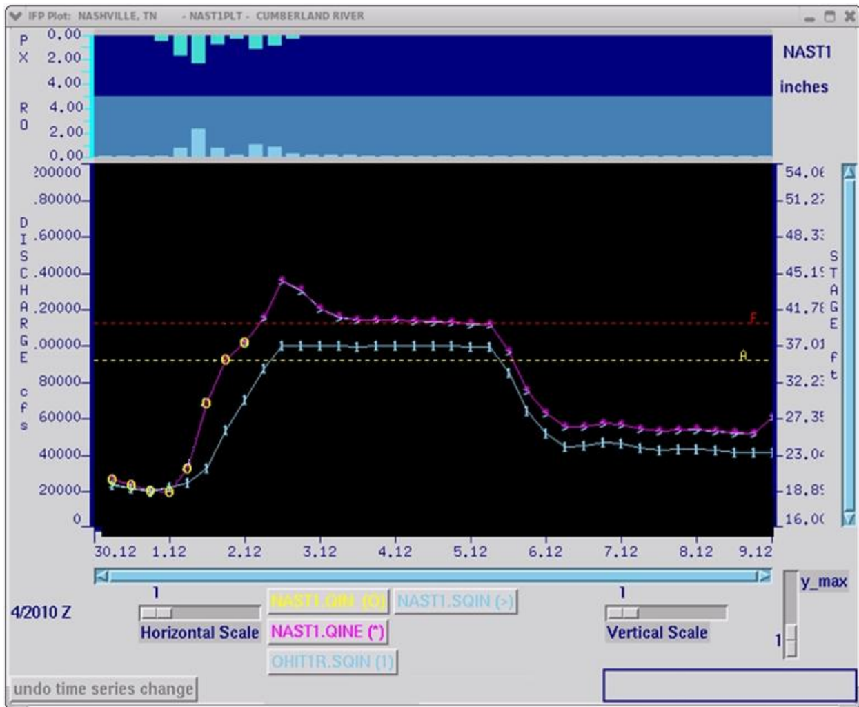
Figure 30: OHRFC Cumberland River model forecasts from Sunday morning. In this figure, release projections provided by USACE LRN for Old Hickory Dam were incorporated into the reservoir model simulation. Observed Old Hickory flows are shown by yellow “O” symbols and extend to 05/02/2010, 1200Z. The blue line with a “1” symbol is the model simulated Old Hickory outflow; the purple line with plotting symbol “*” represents the resulting alternative forecast of river stage at Nashville (using model- simulated, Old Hickory releases).
