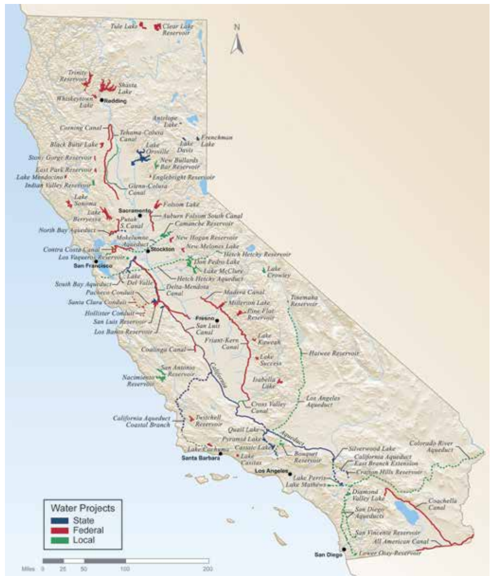
Map showing the water storage and distribution system in California. Source: Courtesy of California Department of Water Resources; CWP 2013
