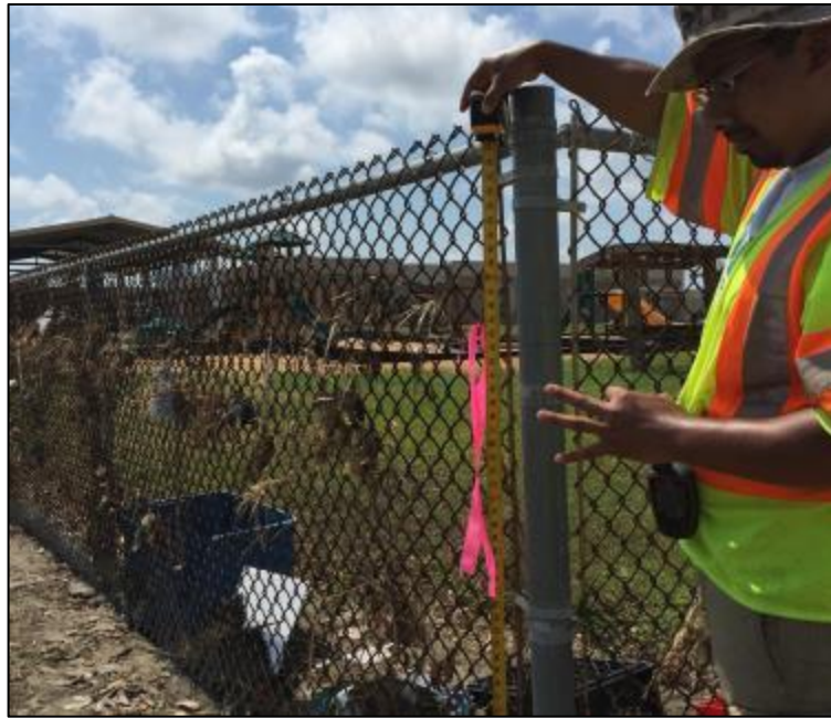
Figure 14: Storm tide high water mark of 3.75 feet above MHHW at Port Aransas High School, Aransas County, TX. Source: USGS Storm Event Viewer, Hurricane Harvey 2017
