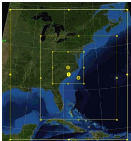
Figure 3.12. WRF domains used for Ernesto simulations: outer domain features 36-km grid spacing, with a 12-km and 4-km middle and innermost domain grid length, respectively.
