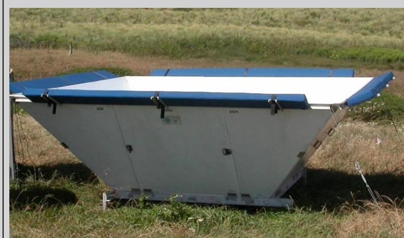
915 MHz phased array wind profiler
