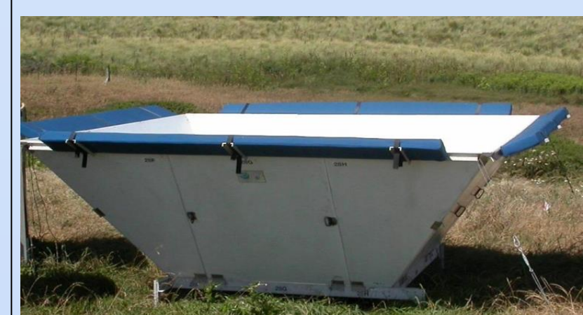
915 MHz phased array wind profiler
