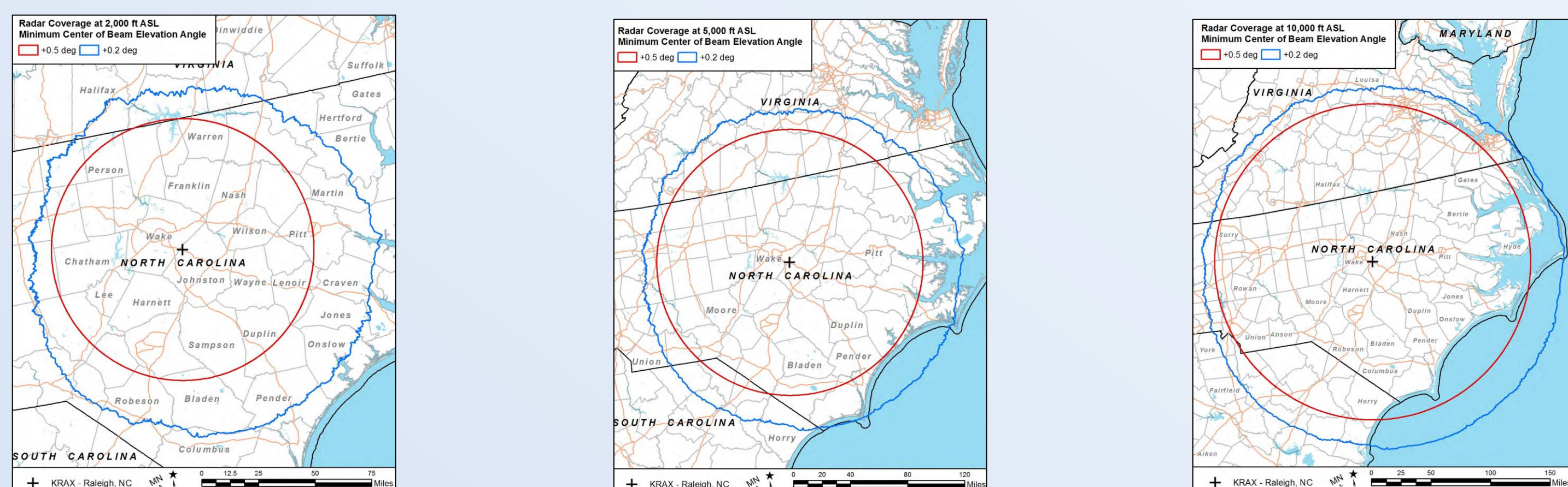
Fig. 2. Comparison of KRAX WSR-88D Radar Coverage at (a) 2,000 ft, (b) 5,000 ft, and (c) 10,000 ft above Site Level for the previous lowest (0.5°) and new lowest supplemental (0.2°) elevation angles (Manidakos and Tarpinian 2019).
