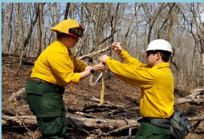
NWS meteorologist Reggie Roakes (right) is assisting Samantha Lopez (left) from the Virginia Division of Wildlife Resources to assess the fuel moisture by weighing fuel sticks.
