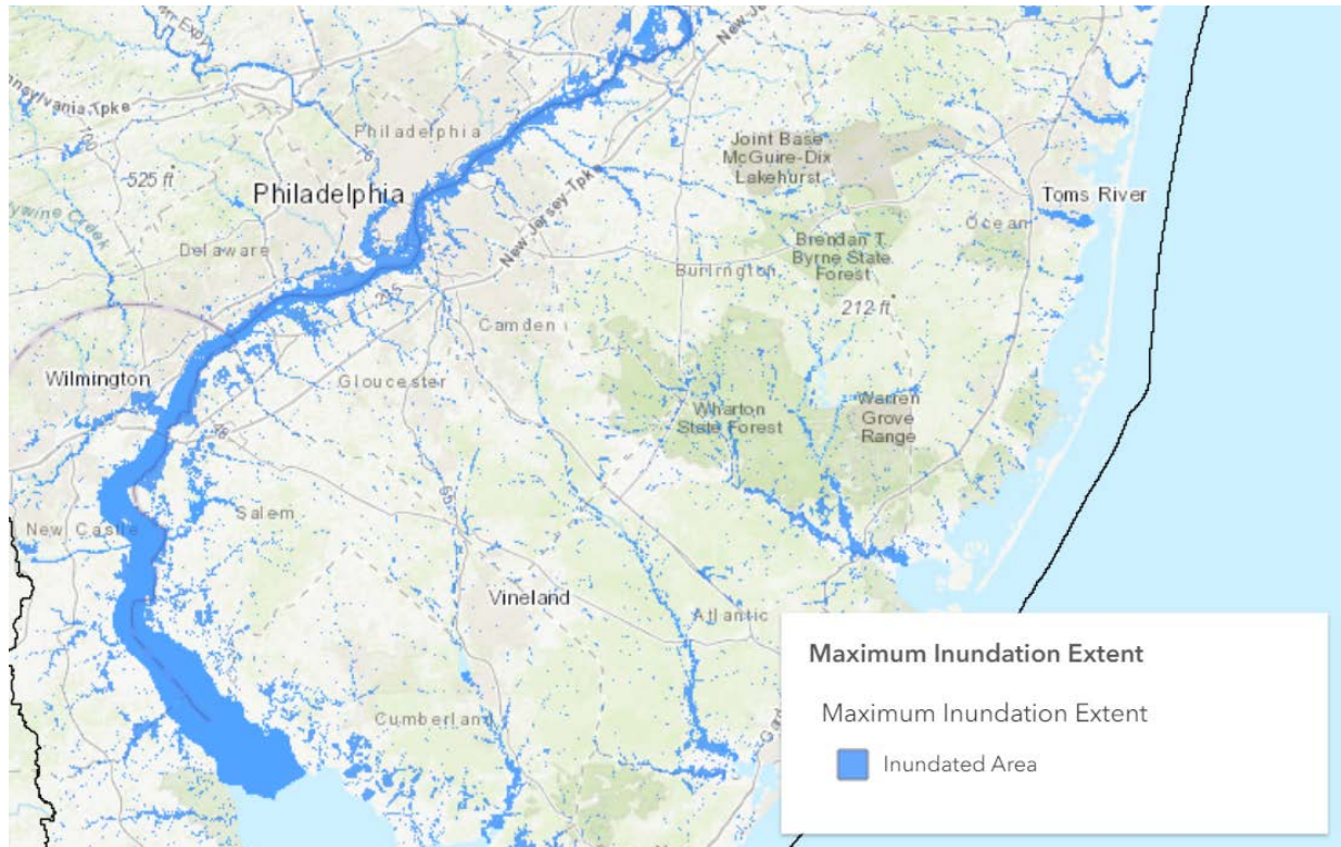
Figure 4. Image of modeled current maximum inundation extent for the lower Delaware Basin.
