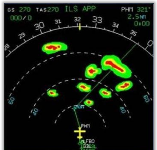
Figure 14 – Same display with range increased from 40 miles to 80 miles.
