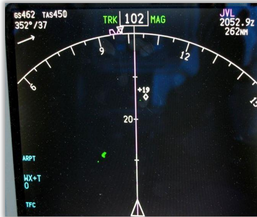
Figure 11- Cockpit weather radar display with the antenna set to auto-tilt (0 degrees) showing a small, weak echo in green, approximately 10 miles to the northwest.
